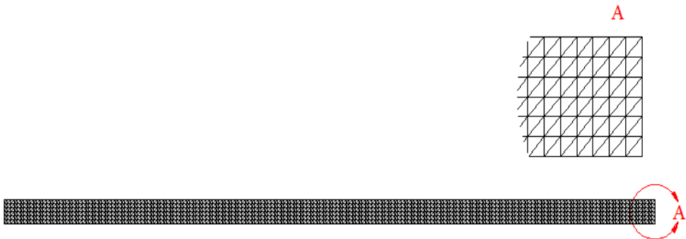
Fig. 4. Mesh for two-dimensional simulations.
